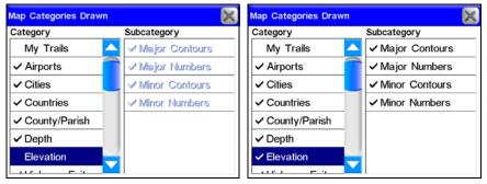
You must turn on Elevation in Categories Drawn to see topo lines. At left, elevation is off; at right the feature is on.
